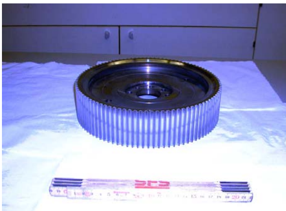
Fig.4 Pulsed Plasma Nitrided Mandrel
